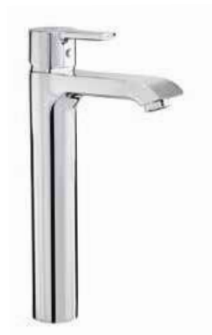
RAK13061 single lever basin mixer XL HR DN 15 ceramic cartridge-K35 aerator M 24 x 1 1/2" high pressure flexible hose with PEX tubes European standard - EN 817
