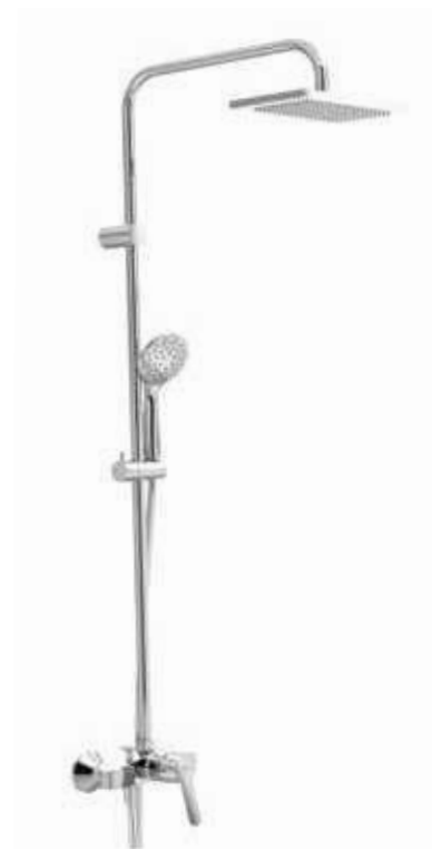
RAK18032 Shower mixer with Dual shower system L-shape L = 1175 mm wall fastening hand and head shower with diverter with 1S hand held shower 1/2 inch ridgeless adjustable shower holder vertically and cylindrically adjustable shower holder shower hose 1/2 x 1/2 inch x 1600mm with fixing kit swivel head shower
