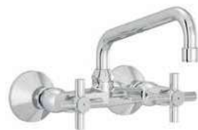
RAK34001 Dual controlled wall mounted sink mixer DN 15 swivel spout aerator M22 x 1 flow class A S- unions 1/2 inch x 3/4 inch European standard- EN200
