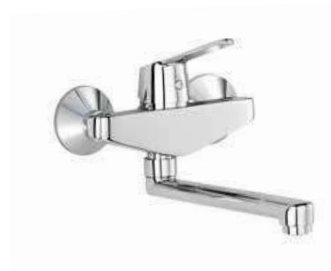
RAK18008 Wall mounted single lever sink mixer DN 15 ceramic cartridge-K35 swivelling (185°) spout l = 200 mm aerator M 24 x 1 flow class A S- unions 1/2 X 3/4 inch European standard- EN 817
