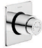
FA01011 Metropole flush valve concealed 32mm single flush with square cover plate
